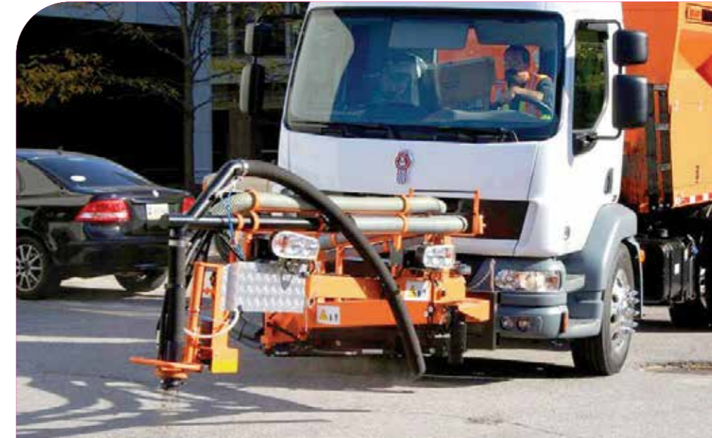
Top: Figure 19 – Base stabilisation with emulsion Bottom: Figure 20 – Spray injection patcher
