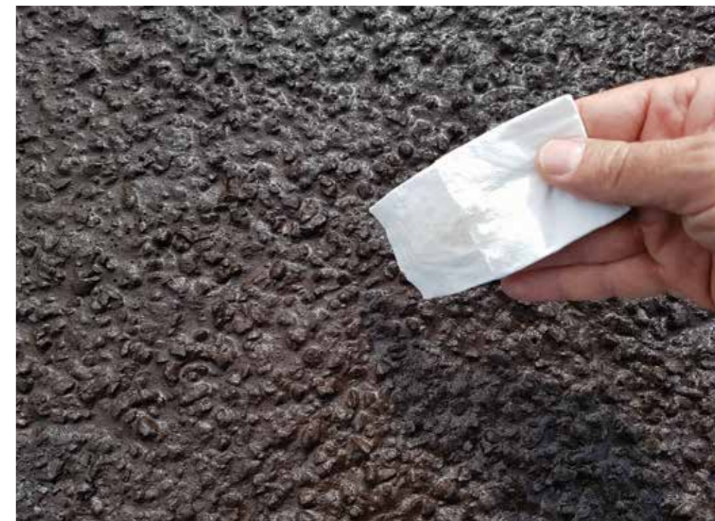
Top: Figure 14 - Polymer modified emulsion for surface dressing Bottom: Figure 15 - Microsurfacing in quick break systems
