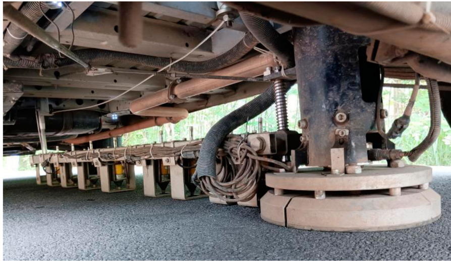
Figure 6. Loading plate and geophones.
