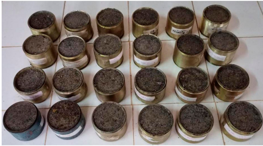
Figure 7. Samples prepared for ITS test.
