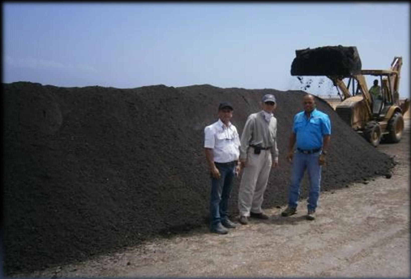
Storage of mix, 48 to 72 hrs to allow moisture content reduction
